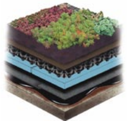
Figure 1. Typical Extensive Green Roof Layers
